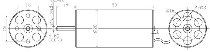
• There are two choices of outer shaft diameter: Dia3.175 or Dia4
